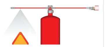
Upon flame impingement or heat the pressurised detection tube which is connected to a cylinder containing the suppression agent ruptures with a burst at the hottest point. The agent is then discharged through the burst hole directly at the heart of the fire.
