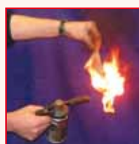
Uncoated fabric under fire conditions
